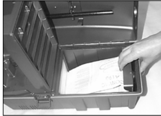
Fig 8. Clip the retainer back into position within the Vacuum Cleaner shell.
