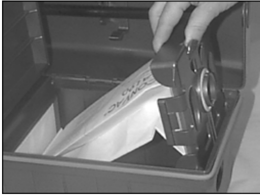
Fig 7. Refit the Retainer with Filter Bag attached.
